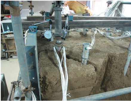
图 3 竖向加载实物图 Fig. 3 Photo of vertical loading device
